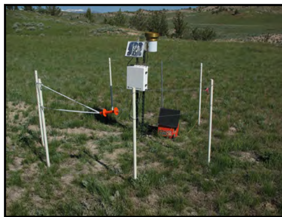
Figure 1. Newly instrumented soil moisture and rainfall recording site near Meeteetse, WY.
